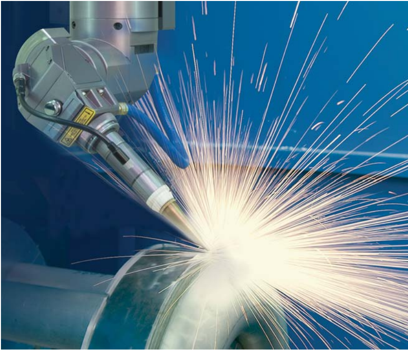
THE LASERDYNE BEAMDIRECTOR 3 DRILLING SHALLOW-ANGLE HOLES ON THE DOME OF A COMBUSTOR ASSEMBLY FOR A BUSINESS JET
