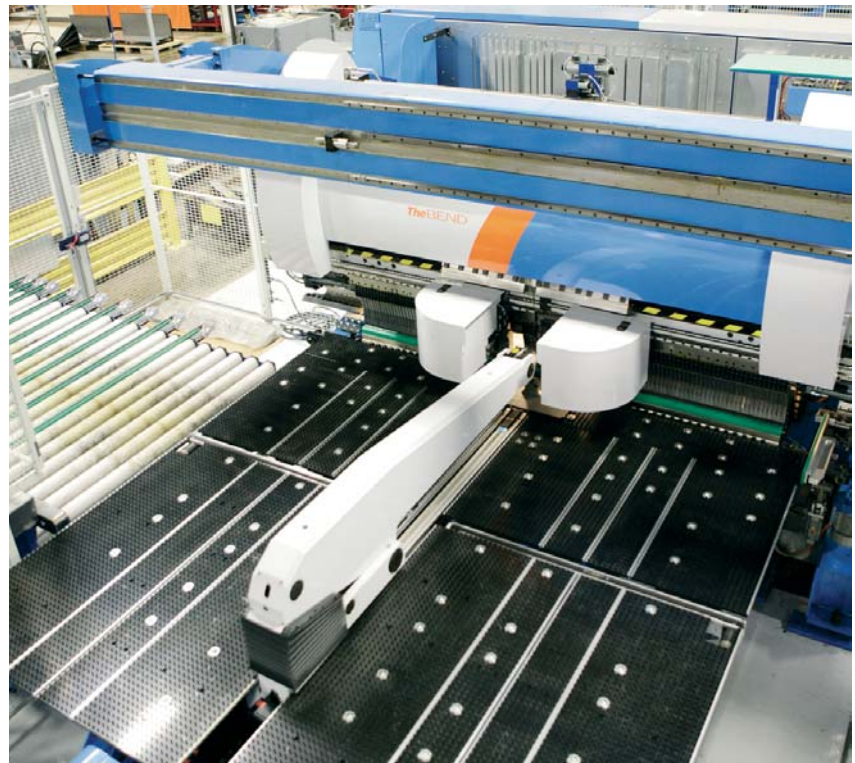
EBe, AUTOMATIC BENDING SYSTEM INSTALLED AT SIEMENS, WEST CHICAGO (IL)
