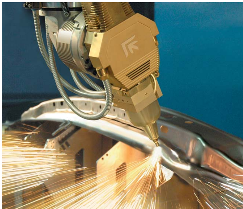
THE PRIMA POWER 3D LASER CUTTING HEAD PROCESSING AN AUTOMOTIVE COMPONENT
