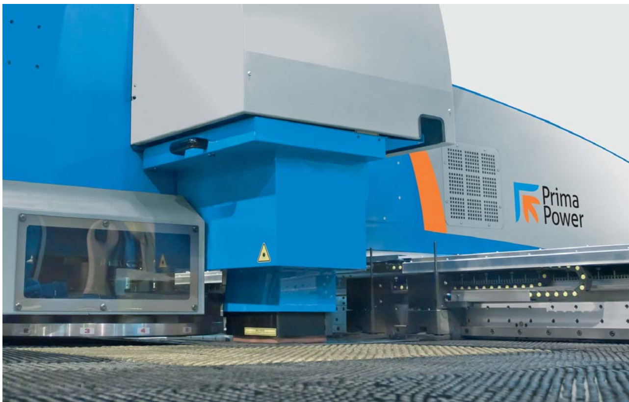
PRIMA POWER LPe COMBINES SERVO-ELECTRIC PUNCHING AND FIBER LASER CUTTING
