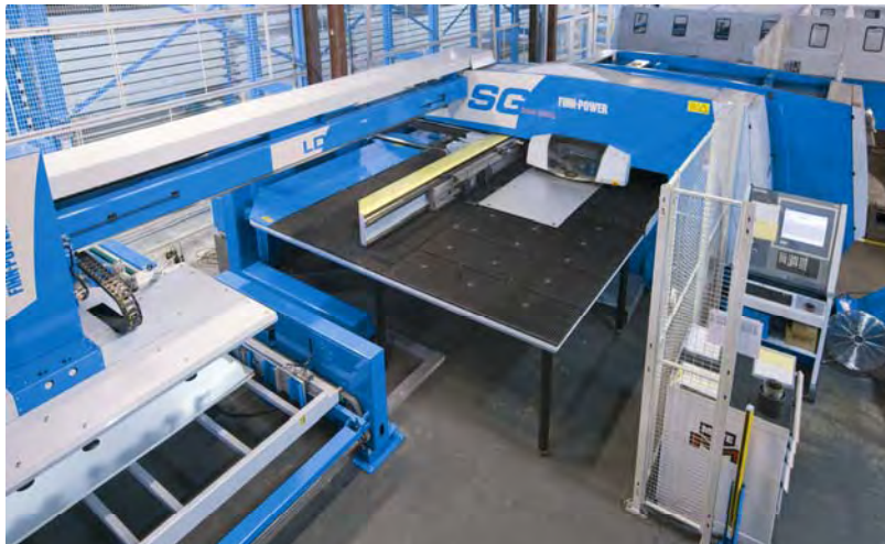
New SG, electrical shearing system
