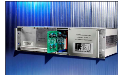
Bogie&stability monitoring control units
